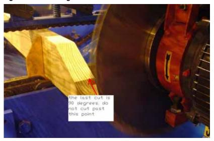
f) Back the board all the way out of the saw using the JOG button. Check to see that all three cuts intercept at the same point.
