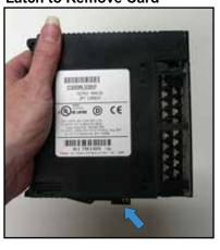
For troubleshooting purposes, you can temporarily switch the suspected bad card with another card of the same type. Use your electrical schematics to determine which slots hold the same type of card.
