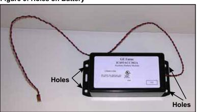
d) Attach the battery to the electrical enclosure using the four (4)  $8-32 \times 1/2$  round head screws included with your kit.
