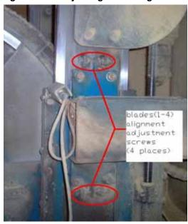
Figure B-15: Adjusting Blade Alignment Jack Screws
