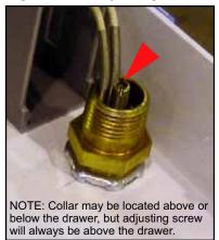
Figure 2-66: Direction to Turn Screw to Increase Temperature
