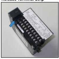
Figure 2-72: Press Release Latch to Remove Card
