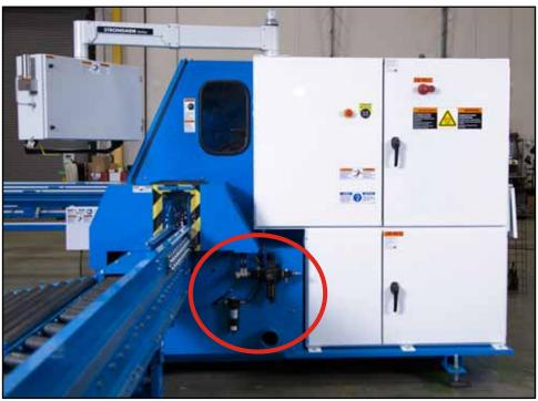
Figure 2-53: Location of Main Filter/Regulator and Cooler Filter
