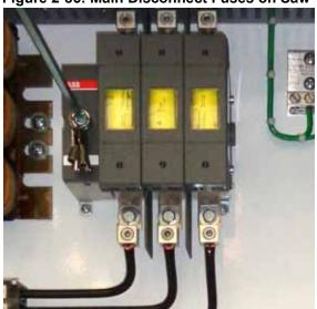
Figure 2-86: Main Disconnect Fuses on Saw
